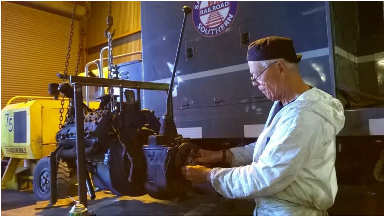
Jim Bays gets the A-6 motorcar's transmission back together
